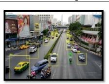
Fig 12: Classification of Two-wheeler and Fourwheeler
